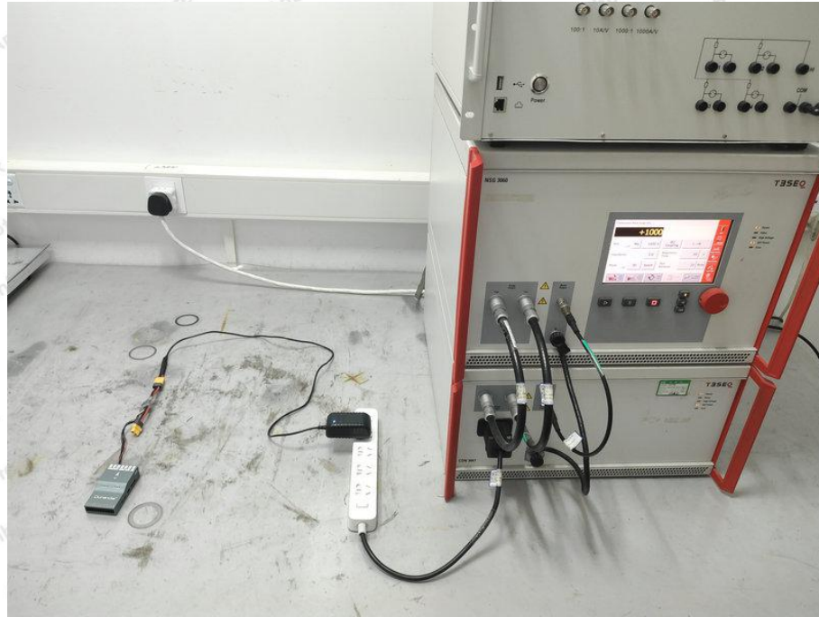
Photo of Surge Immunity Test
