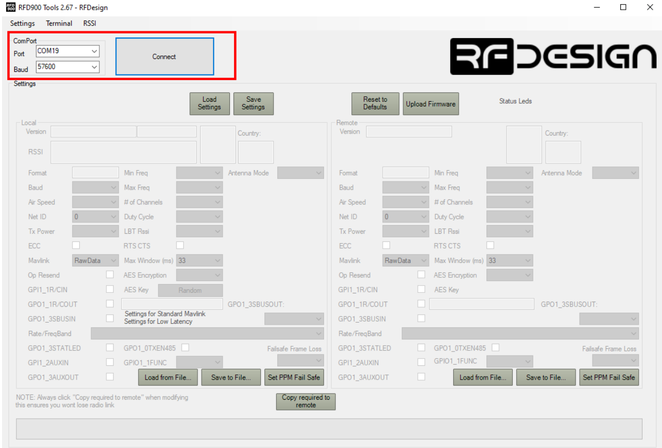
Figure 11: RFD Tools COM port connection
