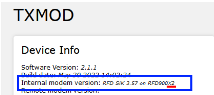
Figure 7: Internal modem hardware version identifier
