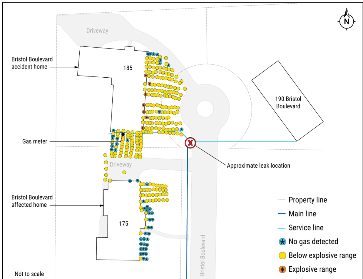
Figure 11. Postaccident bar-hole testing and open-air testing conducted at Bristol Boulevard on January 29, 2024, about 9:15 a.m.
