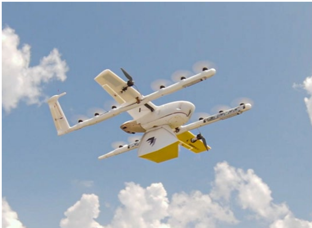
Figure 2.2-4. Wing Hummingbird 7000W-A UA with Package Attached
