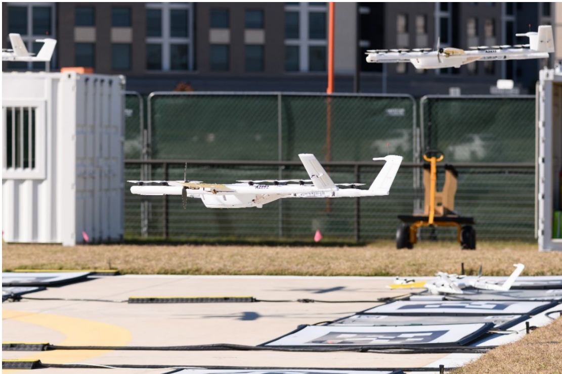
Figure 2.2-5. Wing Hummingbird UA Nest Landing
