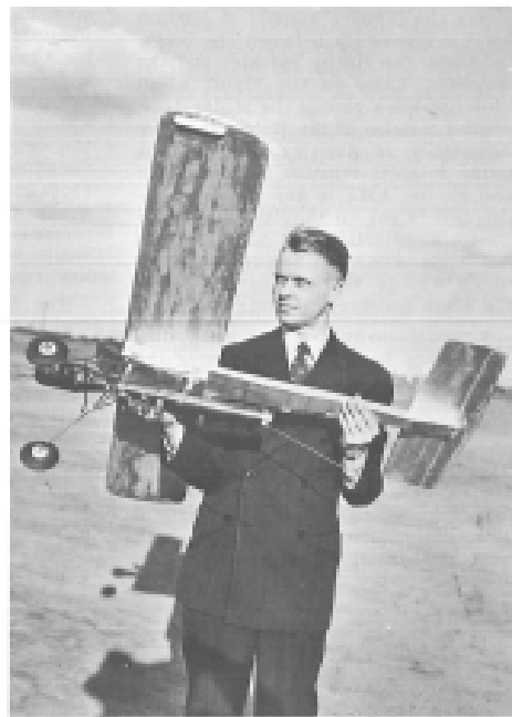
First known Dyno-Jet powered flying model was this control-line shown here. The big model, with much metal, weighed 2 lbs. Developed by Bill Terry.
